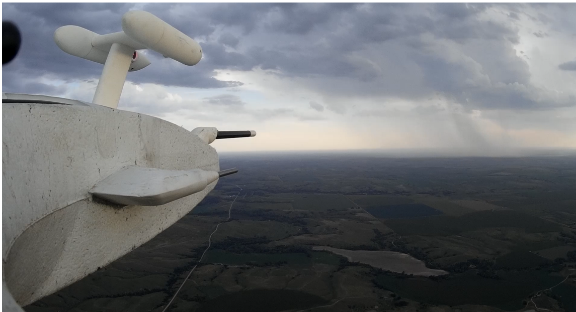
Figure 1. View from the Super RAAVEN uncrewed aircraft of an oncoming cloud. The miniaturized cloud droplet probe (CDP, top), multihole inertial probe (MIP, middle), and inlet to the portable optical particle spectrometer (POPS, bottom) are visible on the nose of the aircraft.
