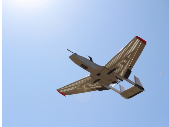
Figure 7. The RAAVEN uncrewed aircraft system, which acts as the Seeding UA for this work.
