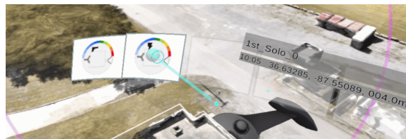
Figure 9. Operator using the context system to quickly select between two close platforms.
