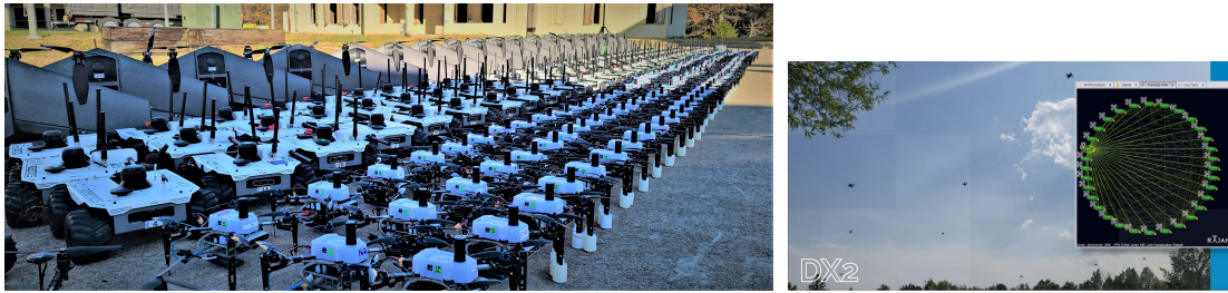
Figure 4. (Left) Rajant ES1 radios are seen mounted to ground vehicles. Aerial vehicles have Rajant DX2 radios mounted underneath. (Right) Mesh radios are shown communicating between IFO platforms during a small-scale field test, as highlighted by Rajant’s network management software.
