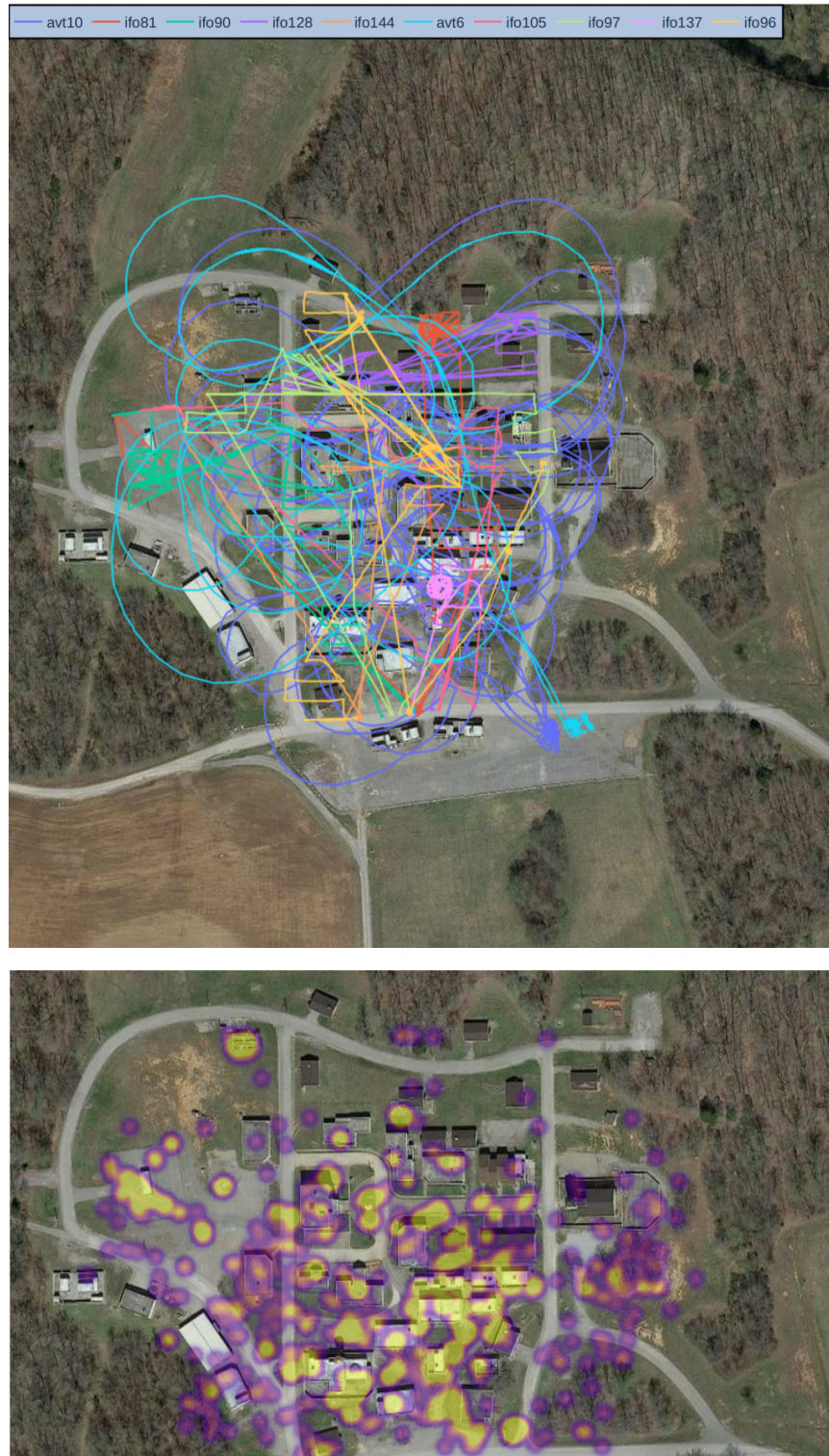
Figure 29. Agent trajectories (top) and coverage (bottom) recorded by NIWC’s orchestration software over the course of run at Fort Campbell during FX-6.
