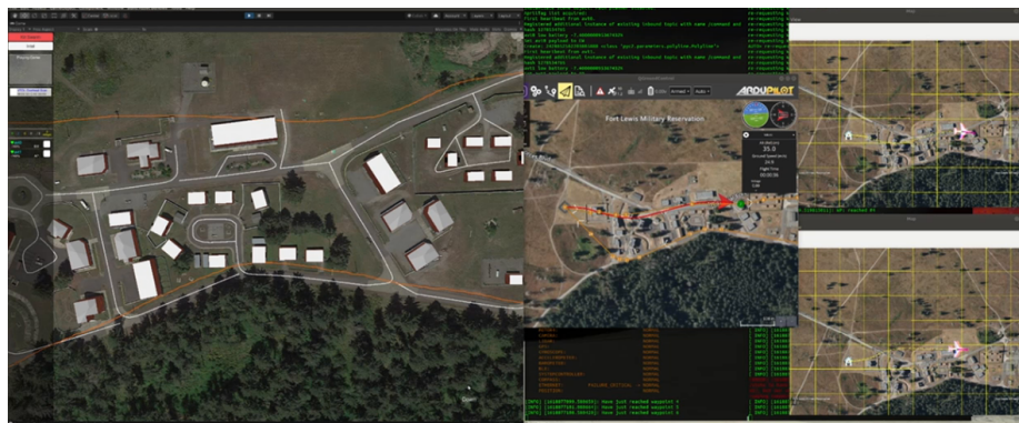
Figure 21. Swarm Engine running alongside the Ardupilot simulator with two simulated AVTs.
