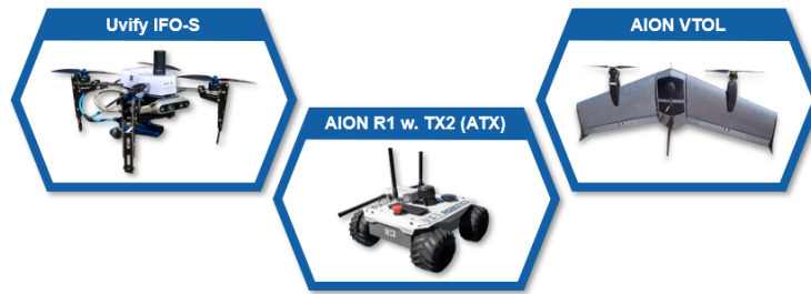
Figure 25. The 274 robotics platforms utilized in FX-6 from left to right: 158 Uvify IFO-S (IFO), 97 Aion R1 (ATX), and 19 Aion (AVT) vertical take-off and landing (VTOL) platforms.
