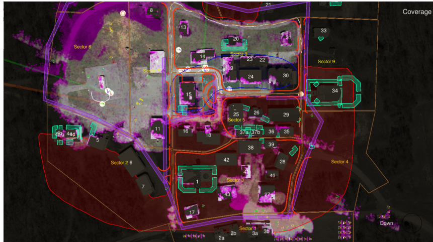
Figure 17. Temporal coverage visualization captured in the course of a joint Northrop Grumman and BBN exercise during the DARPA OFFSET sixth field experiment at Fort Campbell. Dark areas have not yet been examined. Full color areas have current situation awareness. Magenta-colored areas have been previously examined, but the situation data is now stale.
