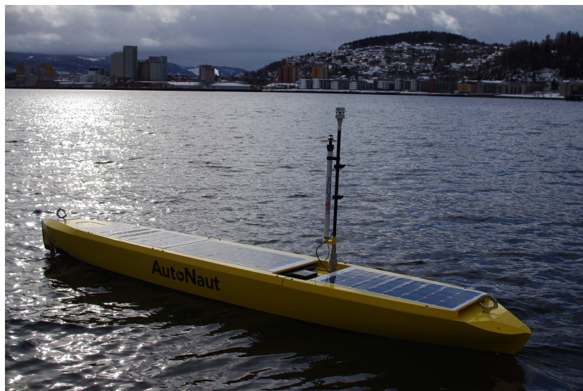
Figure 1. The AutoNaut ASV in Trondheimsjord (Central Norway).
