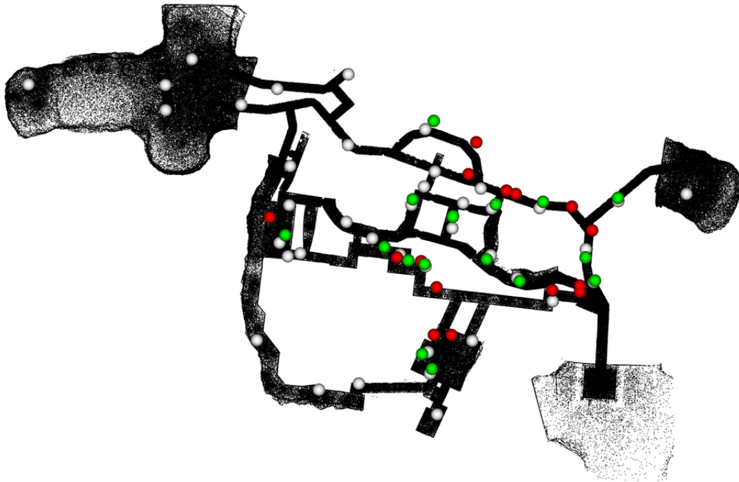
Figure 28. Locations of ground truth artifacts in white, reports that scored in green, and reports that did not score in red, overlaid on ground truth map of the course.
