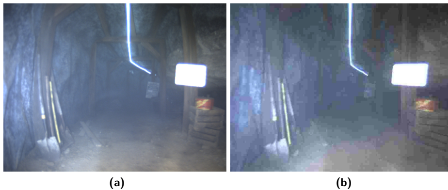
Figure 31. Imagery during robot intervention 2 (RI2). when human supervisor was pushing D01 through the foggy area in the tunnel environment, eventually leading to six additional points. Shown is a comparison of (a) full-resolution FPV imagery onboard the agent and (b) compressed low-resolution FPV imagery transmitted to the human supervisor.
