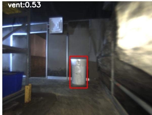
Figure 47. Vent detected and reported by D02 late in mission but missed by the human supervisor due to workload.
