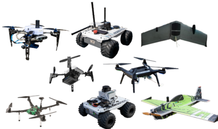
Figure 8. Gallery of OFFSET swarm platforms, including the 3DR Solo (quadcopter), Uvify IFO-S (quadcopter, two configurations), Aion R1 (rover, two configurations), Edge 540XL (fixed-wing), Aion VTOL (VTOL fixed-wing), and ModalAI m500 (quadcopter). (Not shown are multiple platforms deprecated over the course of the OFFSET program.)
