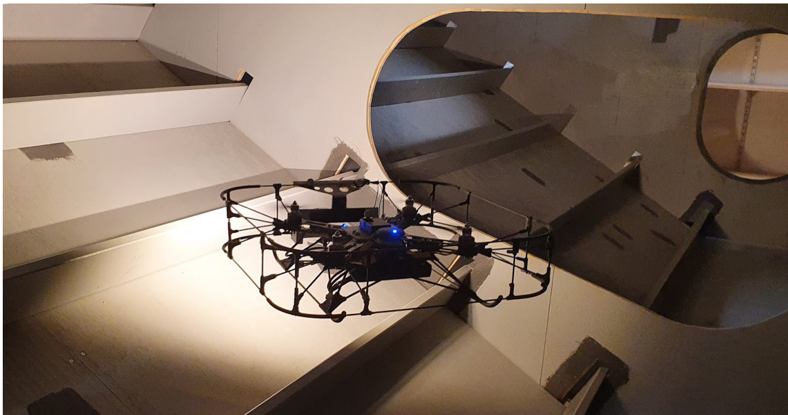
Figure 1. Example of a drone flying in a ballast tank. If equipped with the right sensory equipment accompanied by a high level of autonomy, the drone can replace human surveyors in the hazardous environments present in the ballast tanks of modern marine vessels.
