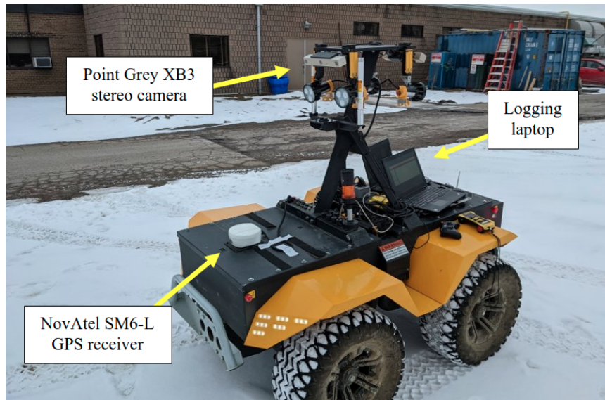
Figure 6. The Clearpath Grizzly Robotic Utility Vehicle used for data collection.
