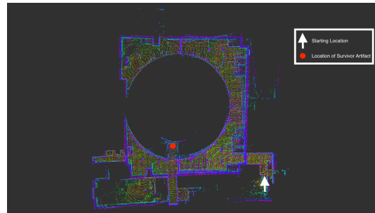
(d) The merged 3D point cloud from two trials on the alpha course.
