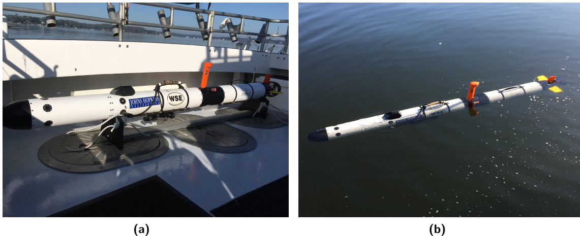
Figure 2. Field trials were conducted with the Johns Hopkins University (JHU) Iver3 autonomous underwater vehicle (AUV) in the Chesapeake Bay, Maryland, USA (OceanServer Technology, Inc., 2016). The JHU Iver3 has a full suite of navigation sensors, including a Doppler velocity log (DVL) and several IMUs (Image credit: Paul Stankiewicz, JHU).
