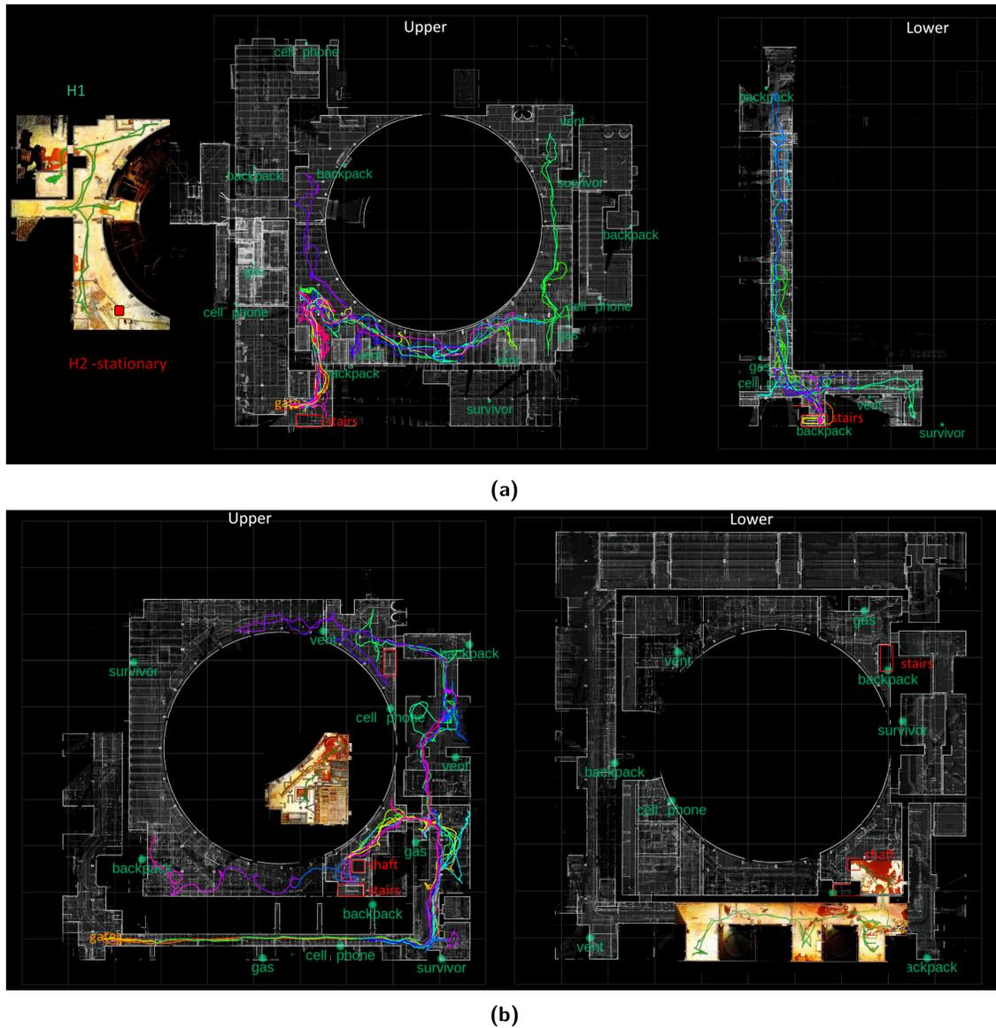
**Figure 24.** Course map and robot trajectories for Urban Circuit event (a) alpha course and (b) beta course. The grey map sections were ground truth data provided by DARPA, with grid cells representing 10 m. The colored map sections, overlaid or adjacent to the grey map, were generated by the UAVs. In the beta course, the UAV flew between the upper and lower levels of the course. The multi-colored trajectories overlaid on the grey map are from the multiple UGV systems.
