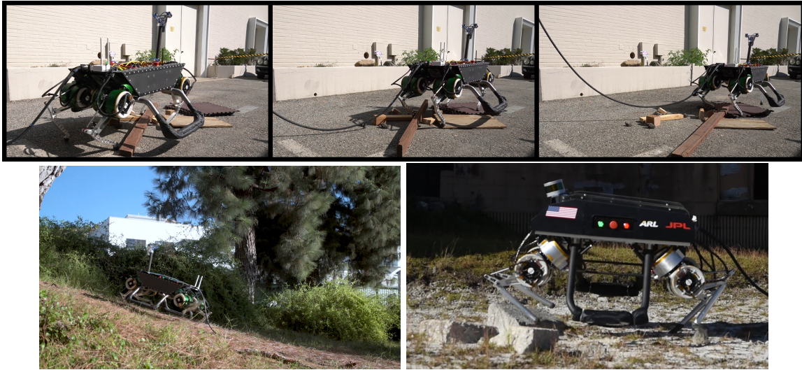
Figure 19. Terrain successfully handled by the reactive locomotion controller
