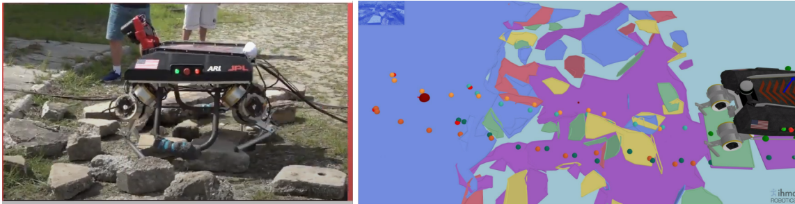
Figure 18. Left: Image of a rock field set up at Camp Lejeune. Right: Using the deliberative controller detailed in a companion paper (Griffin et al., 2021), the robot used lidar data to create a simplified model of the environment, then planned each footstep to traverse the obstacles using an A* planner. The robot then successfully walked over the blocks, up the curb, and onto the inclined concrete slope on the other side.
