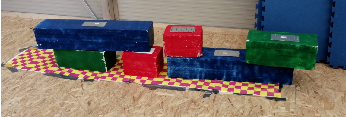
Figure 15. Six brick wall built in an autonomous full-scale MZBIRC 2020 Challenge 2 experiment. Total of three trips between brick stacks and wall were required and all bricks were placed within the boundaries as proposed by the competition.
