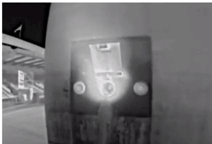
(a) Thermal image of water hitting the fire, just below the opening (water stream shown in lighter grey).
