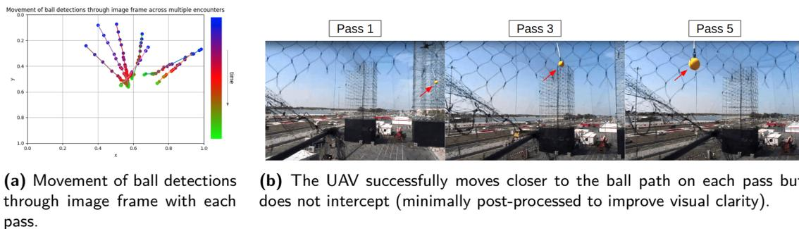
**(a)** Movement of ball detections through image frame with each pass. **(b)** The UAV successfully moves closer to the ball path on each pass but does not intercept (minimally post-processed to improve visual clarity).
