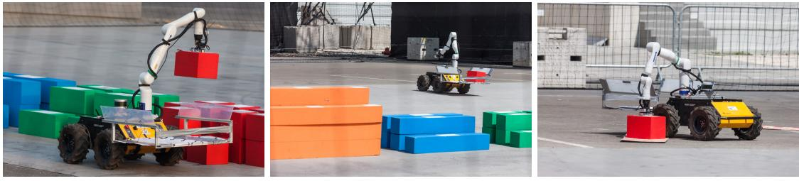
**(a)** Loading a red brick into the cargo bay    **(b)** Searching for the checkered pattern    **(c)** Successful placement of the red brick
