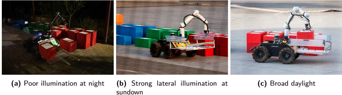
**Figure 20.** The visual servoing and brick grasping procedures have been tested under a variety of lighting conditions, to ensure a robust performance throughout the entire competition day.
