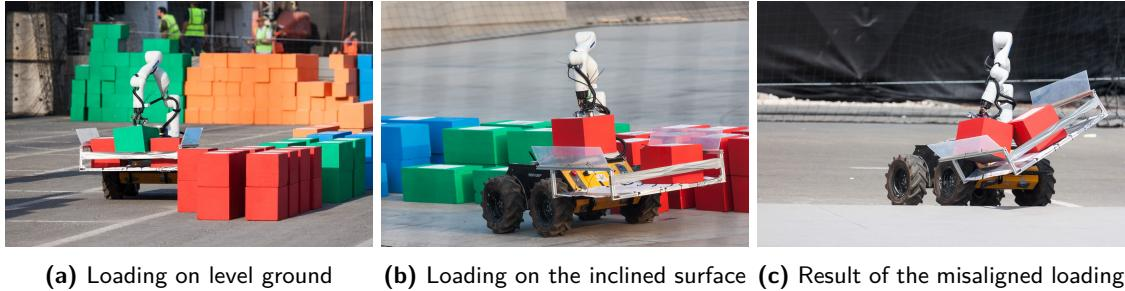
(a) Loading on level ground    (b) Loading on the inclined surface    (c) Result of the misaligned loading
