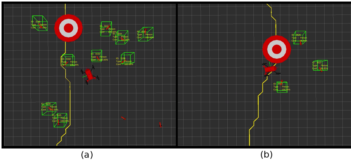
Figure 6. Simulated environment used for testing, illustrating crowd densities of 10 \text{ m}^2 (a) and 25 \text{ m}^2 (b) per agent on a 1 \times 1 \text{ m} grid. The long-term planner's reference path is shown in yellow with the current waypoint as a target. Simulated optimal reciprocal collision avoidance (ORCA) agents are shown as red arrows, with green bounding boxes highlighting agents that the robot is currently tracking.
