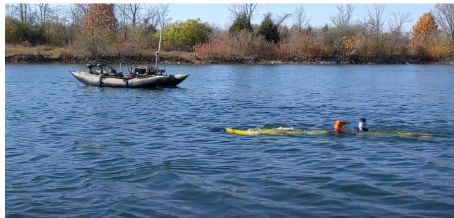
Figure 2. Experimental platforms used in this paper: a custom autonomous surface vehicle with differential steering and an Oceanserver Iver3 autonomous underwater vehicle.
