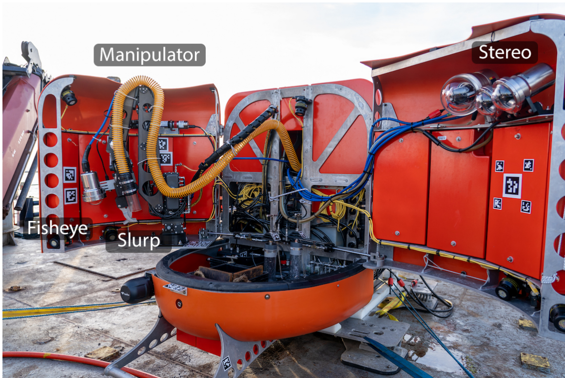
Figure 13. The NUI vehicle is outfitted with clam shell doors that can be closed to reduce drag when cruising and opened to perform manipulation tasks. The manipulator is mounted to the starboard door and the stereo cameras are mounted to the port door.
