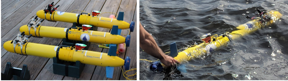
Figure 7. Photograph of the fleet of three Bluefin SandShark AUVs, named Platypus , Wombat , and Quokka (left), outfitted with the OWTT-iUSBL payload; Quokka being hand-deployed dockside (right).
