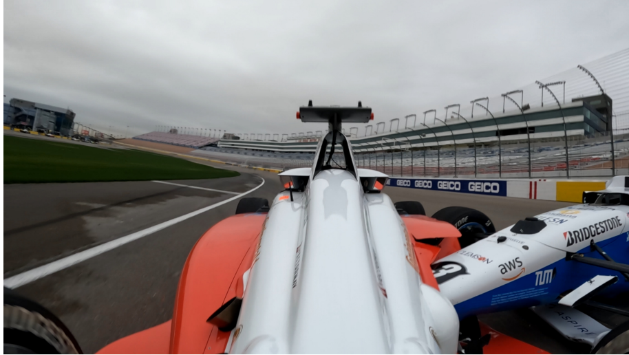
Figure 15. Onboard image from the first known major autonomous, multiagent, head-to-head collision. The competition-style run had both vehicles acting as both Defender and Attacker. In this instant, the opponent AV-21 was attempting an overtake; however, when doing so, the vehicle commanded a very sharp acceleration and lost traction. This resulted in the vehicle spinning out of control and piercing the side of the AV-21. The resulting damage included a fried battery isolator, a destroyed alternator, torn timing belt, pierced side pod, several fuel injectors, a severed engine wiring loom, numerous severed fuel and oil lines, destroyed coolant tubes, and more. To repair the damage, the entire vehicle was disassembled, including removing the transmission and engine, then disassembling the cockpit and autonomy hardware suite. The vehicle was repaired and running again 48 hours later, in time for the competition the next day.
