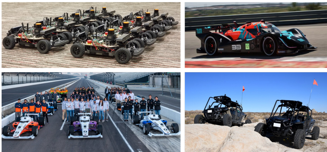
Figure 2. Examples of real-world autonomous racing competitions. (Top left) F1 TENTH, using a 1:10 scaled vehicle. (Top right) ROBORACE, using a full-scale electric race car. (Bottom left) Indy Autonomous Challenge (IAC), using a Dallara AV-21 retrofitted Indy Lights class chassis. (Bottom right) DARPA-RACER program, using autonomous ground combat vehicles in unstructured off-road terrain at speeds.
