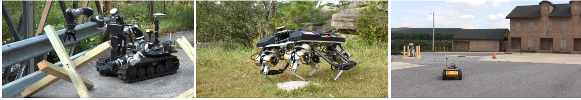
Figure 1. Left: RoMan clearing Czech hedgehog debris. Center: LLAMA taking a step over a boulder. Right: Husky navigating to a gas pump.
