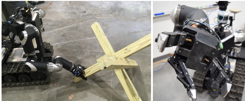
Figure 12. Left: RoMan platform grasping a “Czech Hedgehog” anti vehicle barrier prior to a drag behavior. Failure to account for the motion of the grasp point relative to the ground support contacts during lifting motion results in a large torque being exerted on the gripper about the Y axis of the FLU robot frame. Right: Broken proximal joint on digit 3 of a Robotiq 3-finger gripper after heavy object lift exceeded safe torque levels.
