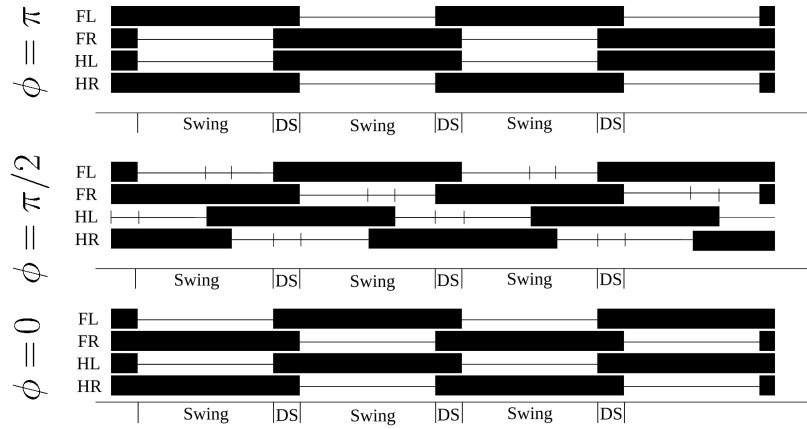
Figure 6. Illustration of the different timings used to define the different gaits of the robot. The top gait is a trot, the middle is an amble, and the bottom is a pace.
