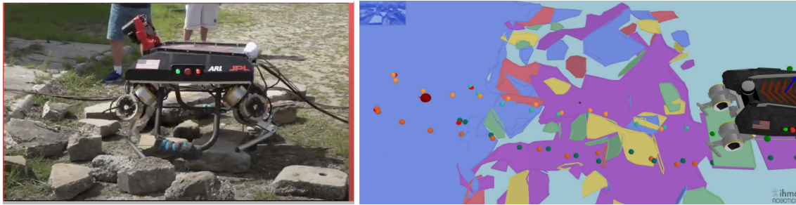
Figure 22. Image of the rock field set up at Camp Lejeune. The robot used LIDAR data to model the environment using the approach presented in Section 3 and planned the contacts using the A* planner in Section 4, shown on the right in the figure. The robot then successfully walked over the blocks, up the curb, and onto the inclined concrete on the other side.
