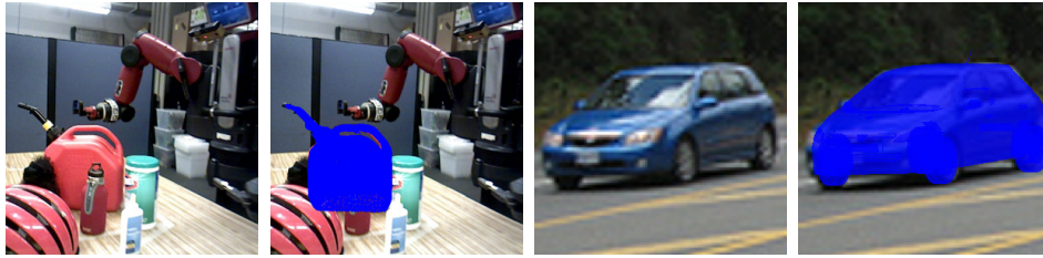
Figure 1. Overview of approach. Given a single RGB image of an object (first and third columns), we estimate its 6-DoF pose. The corresponding CAD model is overlaid on the image (second and fourth columns) using the estimated pose. Our method deals with both instance-based (left pair) and class-based scenarios (right pair).
