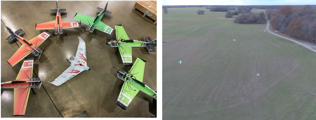
Figure 24. The photo on the left shows the six aerobatic fixed-wing vehicles fabricated to support multi-vehicle operations. The still on the right shows an instance of three aerobatic fixed wings flying in close proximity during OFFSET Field Exercise 6.
