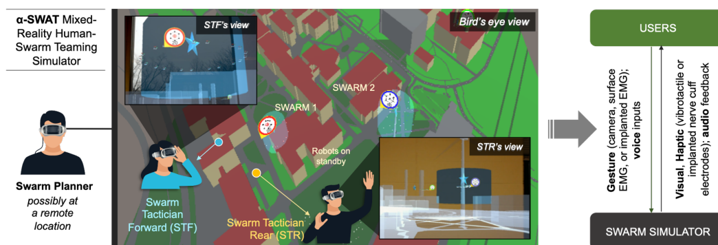
Figure 1. Conceptual illustration of the multimodal visuo-sensorimotor interface for human-swarm interface. Users—Swarm Planner (SP), Swarm Tactician-Rear (STR), and Swarm Tactician-Forward (STF)—communicate and collaborate with the swarm at the levels of individual robot, subset, and the entire swarm via vision- and sensorimotor-based interaction.
