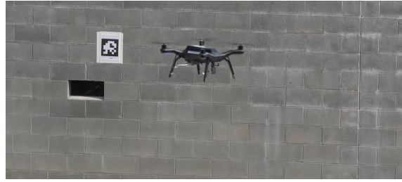
Figure 2. A Building surveillance task, during which a UAV detects the artifact. Photo courtesy of DARPA.
