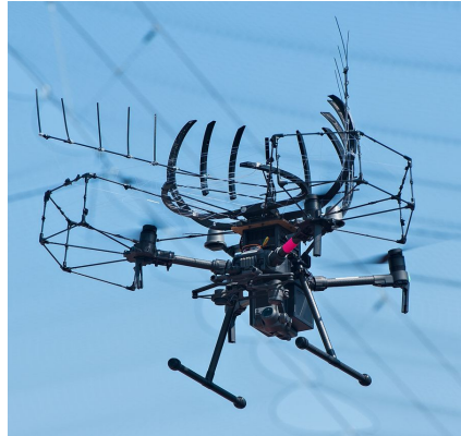
Figure 6. The complete proposed platform, with the gripper and all protections included in the real competition environment.
