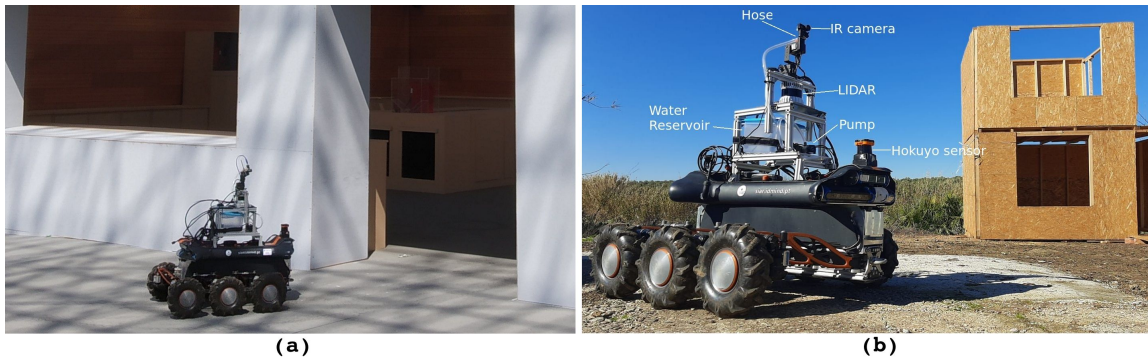
Figure 2. The ground platform used for Challenge 3.(a) Showing performance in the scenario of MBZIRC (b) Deploy of onboard sensors and Water Extinguishing System
