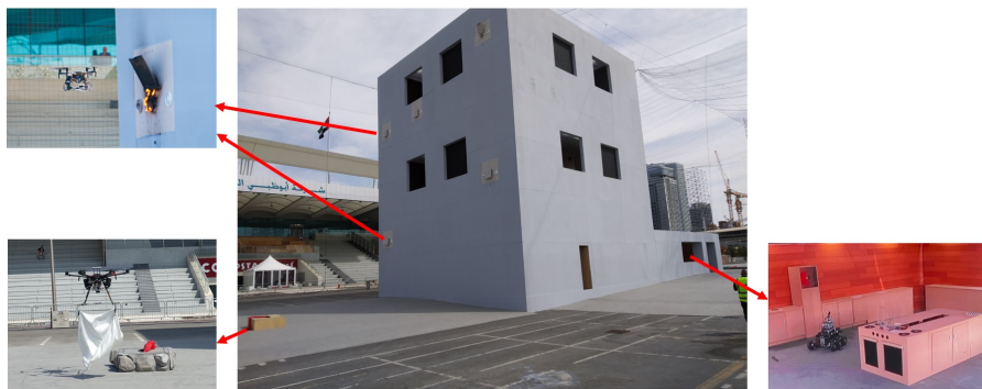
Figure 1. Arena of Challenge 3. There are simulated fires on the facades of the building (top-left), and inside the building (down, right), located on the ground, first and second floor (to be suppressed with water). There are also fires located on the ground outside (down, left) that need to be suppressed with a blanket.
