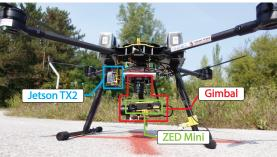
Figure 2. Target intercept scenario at MBZIRC 2020 challenge (left, courtesy of http://mbzirc.com/) and custom made Kopterworx Eagle UAV used by LARICS team at the competition (right).
