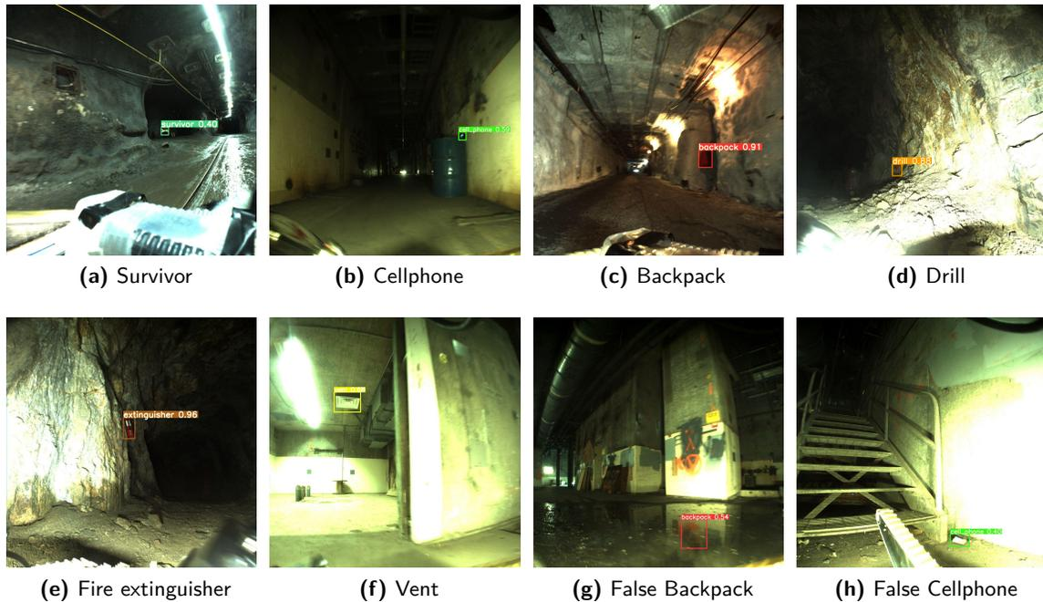
**Figure 7.** Detection of all object classes during the challenge. Two false positives are depicted, Backpack as the red sign in water reflection and cellphone as a piece of paper.
