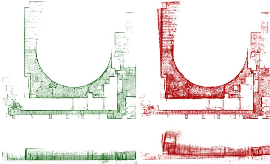
**Figure 9.** Maps of the Beta course obtained from our localization pipeline (left, green) and from the A-LOAM algorithm (right, red). The sensor data come from the Husky robot during the second Beta run. The top row presents a top-down view, the bottom shows side-views of the resulting maps.
