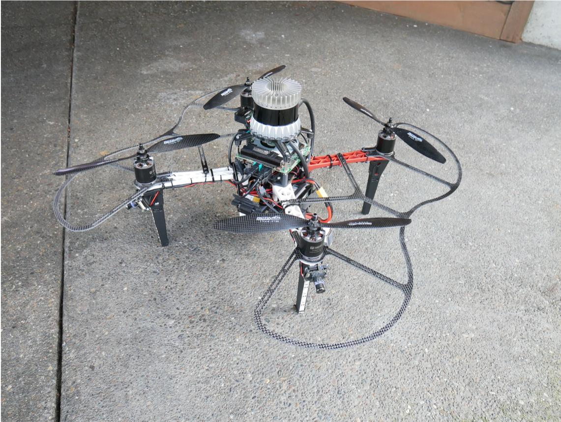
**Figure 5.** One drone platform with propeller guards and Ouster sensor on top.
