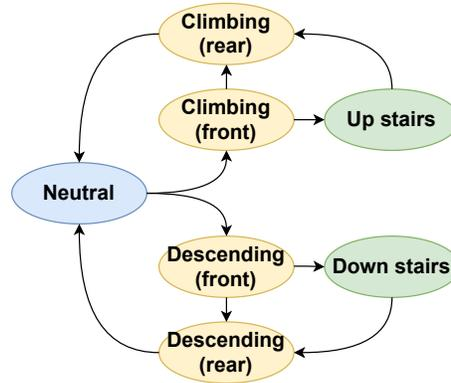
**Figure 11.** Finite state machine for controlling flippers of the Absolem platform, capable of traversing difficult obstacles and stairs. Blue and green states signify longer lasting modes, whereas yellow states are short lasting.
