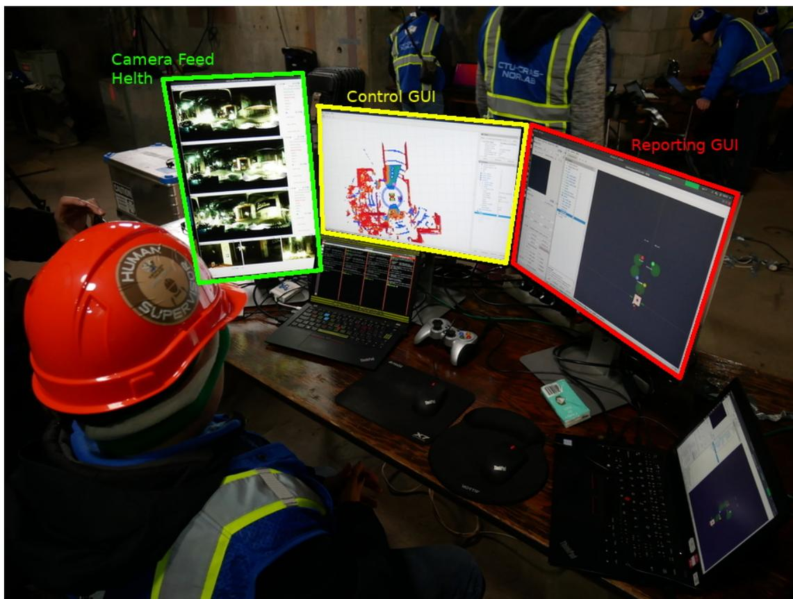
**Figure 12.** The base station and its user interface used in the Urban circuit event.
