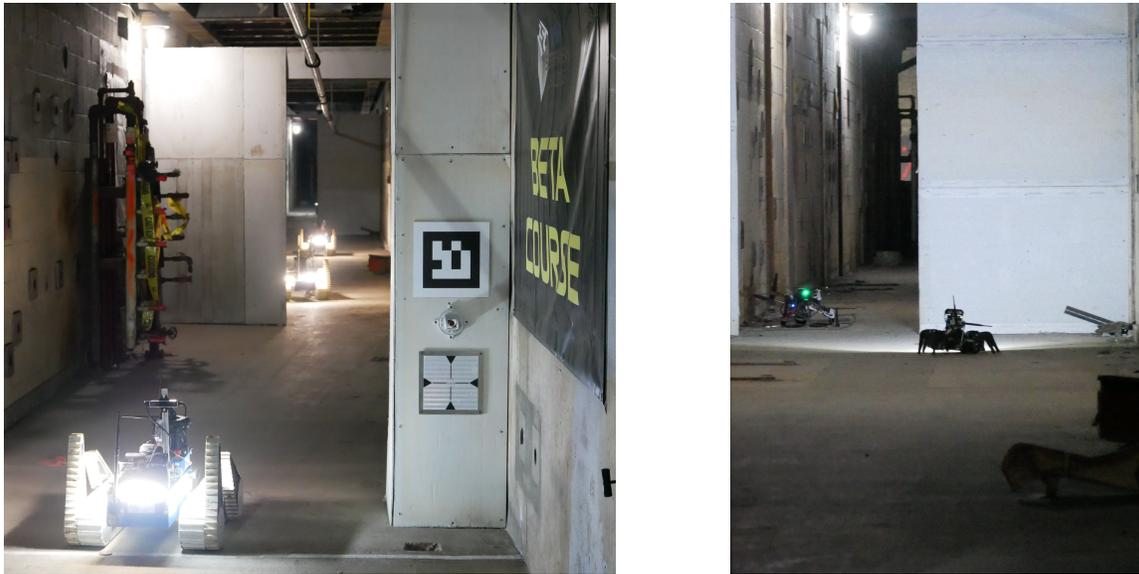
**Figure 1.** Team of ground robots exploring entry hallway (left) and crashed UAV being observed by hexapod (right) during DARPA SubT at Satsop nuclear powerplant.
