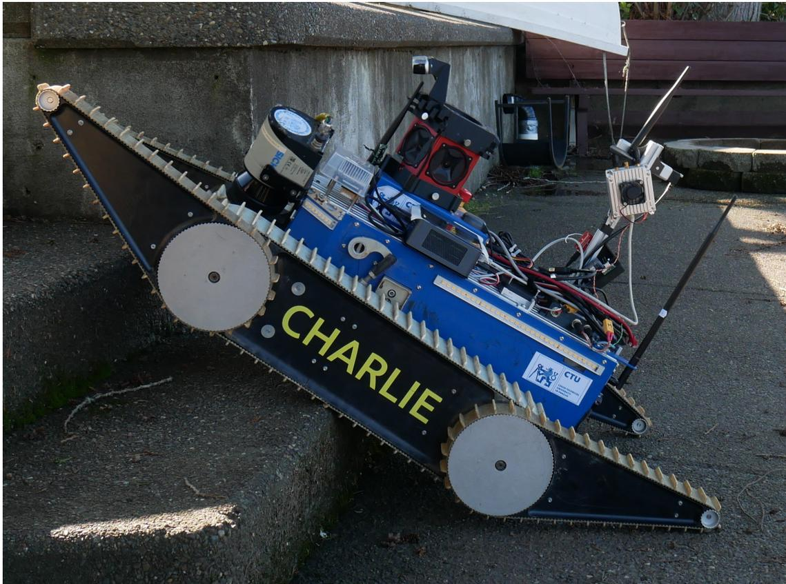
**Figure 3.** Absolem climbing concrete stairs using extended flippers.
