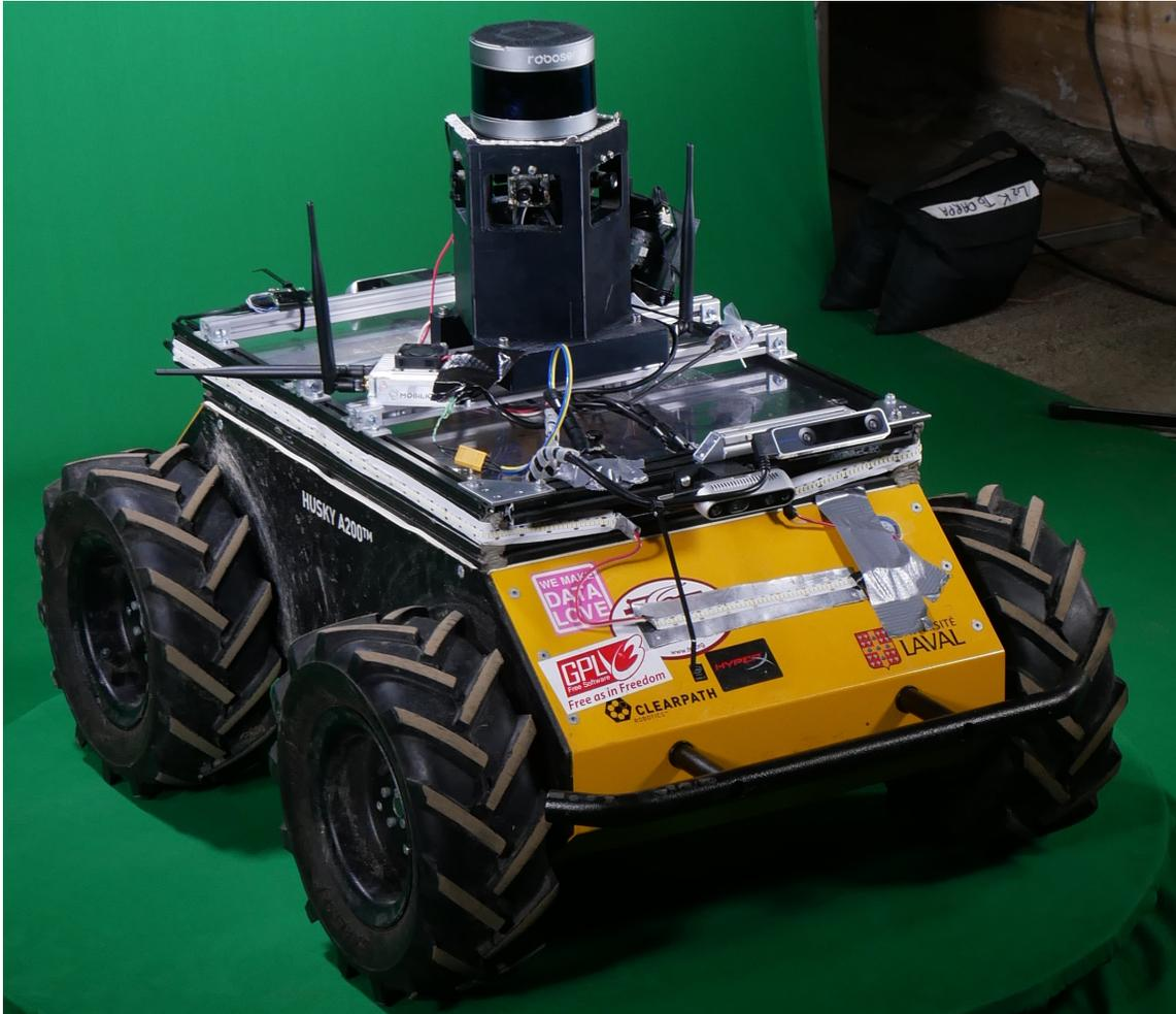
**Figure 2.** The Husky platform with a Robosense lidar on top of a sensory tower which houses five cameras.
