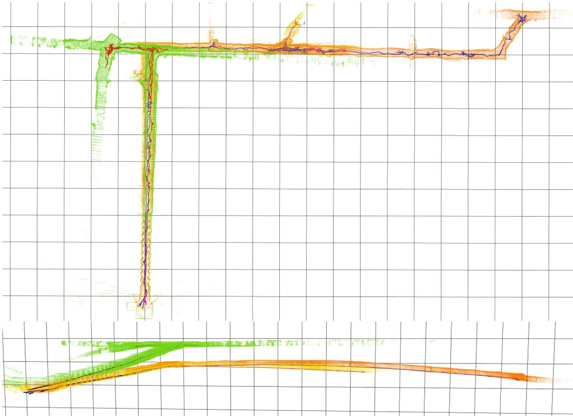
**Figure 16.** Top and side view of a Run 4 in Tunnel circuit. Slight misalignment of robots at the beginning causes visible error in mapping clearly visible at T junction. Bottom image shows heavy drift in localization and map bending. 10-m grid
