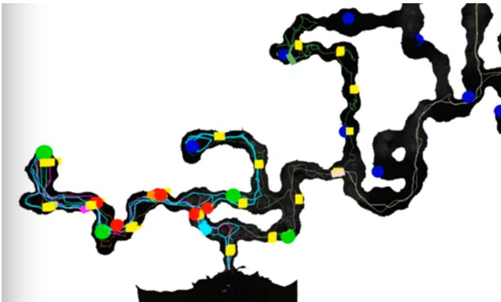
**Figure 19. Path trace of a scored competition run.** Colored lines are traces of individual robots. Blue circles are ground truth artifact positions. Green circles are scored artifacts. Red circles are unsuccessful artifact reports (wrong position or class). Yellow rectangles are dropped communication notes.
