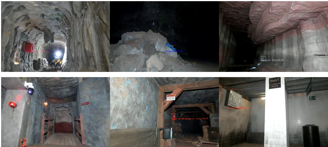
Figure 24. Example object detections from the UGVs.
