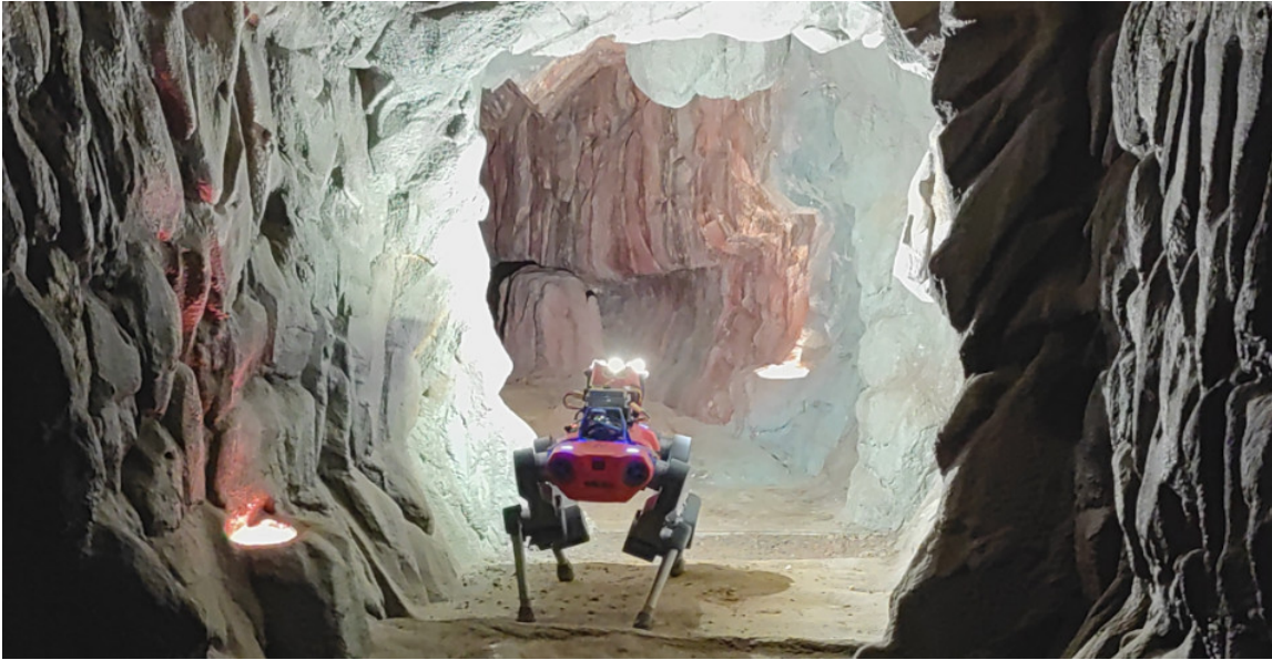
Figure 1. Team CERBERUS won the DARPA Subterranean Challenge Finals with four ANYmal quadrupeds deployed during the Prize Run. The navigation planner presented in this work guided all four robots safely during the hour-long mission.
