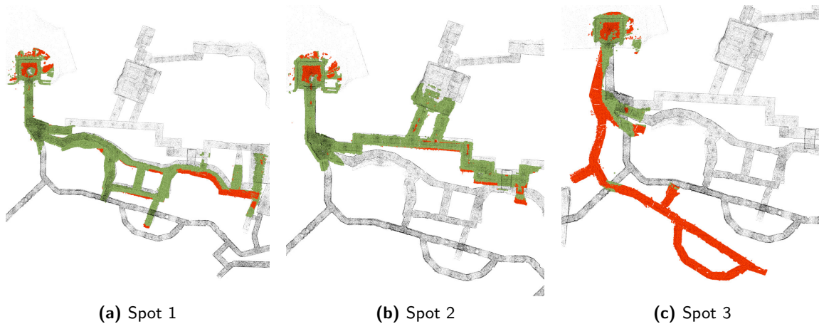
Figure 25. Map coverage and outliers visualized for each robot deployed in the Post-event testing. Ground truth is black, inlier points are colored green, and outlier points are red.
