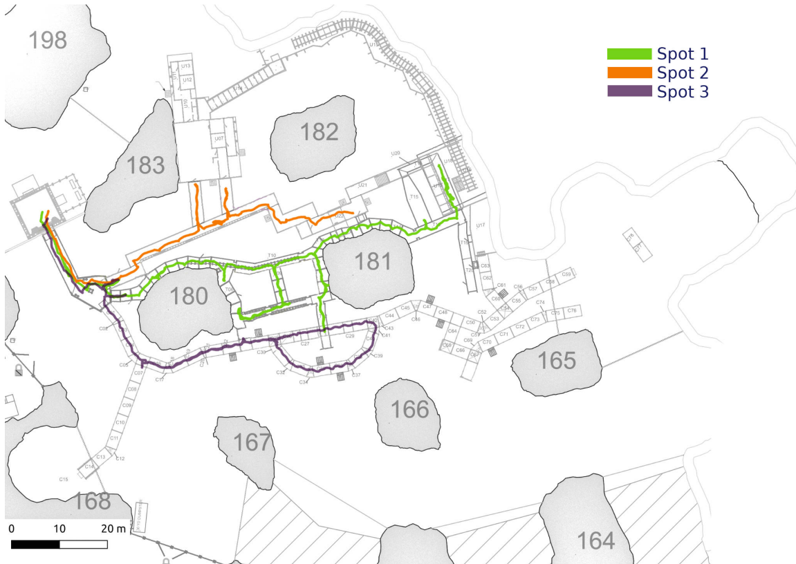
Figure 24. Paths taken by the quadruped robots in the fully autonomous mission of the Post-event testing scenario. The mapping error is captured in Figure 26.
