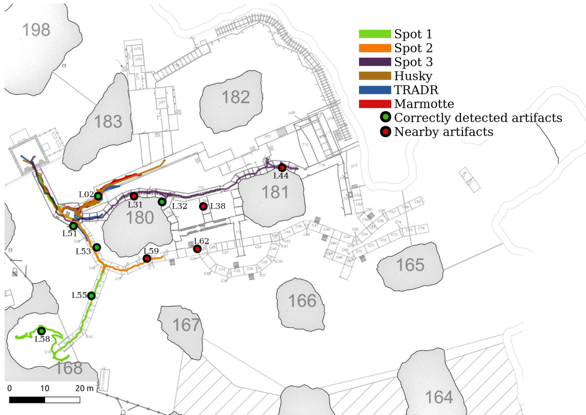
Figure 21. Artifacts detected by the ground robots and paths showing where the UGVs traversed through the Final circuit of the Systems track. The mapping error is captured in Figure 23. The small red disks denote nearby not correctly detected artifacts.
