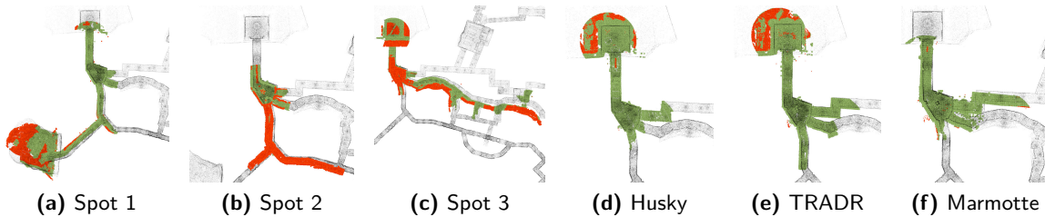
Figure 22. Map coverage and outliers are visualized for each ground robot deployed in the Final circuit of the Systems track. Ground truth is black, inlier points are colored green, and outlier points are red.
