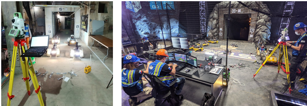
Figure 3. The robots line up in front of the entry gate to the mission area for (left) the Urban circuit and (right) the Final circuit at the beginning of the run. The coordinate frame of the robot is initialized using the Leica TS-16 total station with a laptop computer mount and the retroreflective markers attached to the robot and entry gate.
