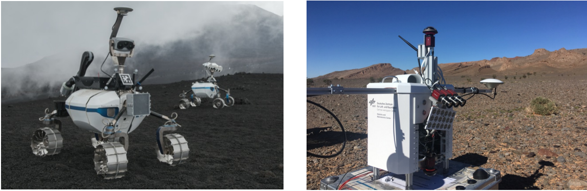
Figure 2. Pictures of the Lightweight Rover Unit (LRU) rovers on Mt. Etna (left) and the Sensor Unit for Planetary Exploration Rovers (SUPER) handheld system in the Morocco desert (right).
