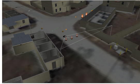
(b) The world state after the robot completed its goal. The initial command “Drive to the cone” was ambiguous. The inverse semantics process generated the disambiguating question “Did you mean the leftmost cone, the middle cone, or the rightmost cone?”. The reply “the rightmost cone” produced the illustrated and achieved goal state.
