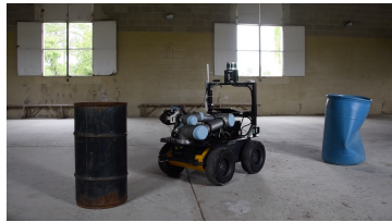
(d) The robot is provided with the instruction “push the full barrel” which is now ambiguous because after interactive estimation it no longer considers “the leftmost barrel” as being full.
