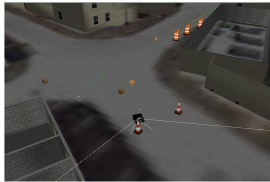
(d) The world state after the robot completed its goal. The initial command “Drive to the cone” was ambiguous. The inverse semantics process generated the disambiguating question “Did you mean the left cone or the rightmost cone?”. The reply “the rightmost cone” produced the illustrated and achieved goal state.
