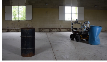
(b) The robot deliberately interacts with the barrel to the robot’s left given the robot instruction “push the leftmost barrel”.
