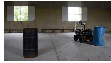
(c) The robot states “the fact the leftmost barrel is full is inconsistent with the world model” after estimating the semantic state as being inconsistent with the world model. The robot also internally updates its representation of that object.
